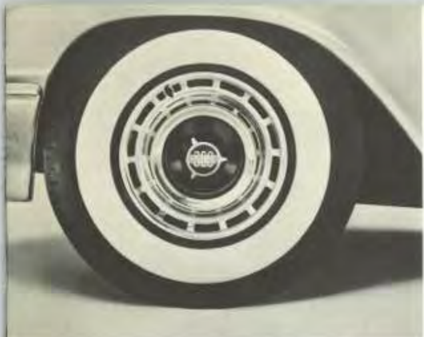
New 15-inch wheels, fitted with sports-tread tires and ventilated wheel covers, greatly improve brake cooling . . . cut brake fading.
