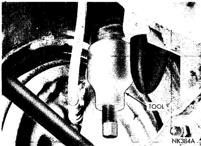
Fig. 20—Removing Upper Ball Joint Stud (Chrysler)
