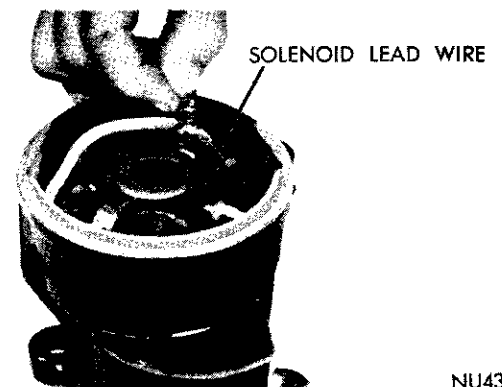
Fig. 3—Unwinding or Winding Solenoid Lead Wire
