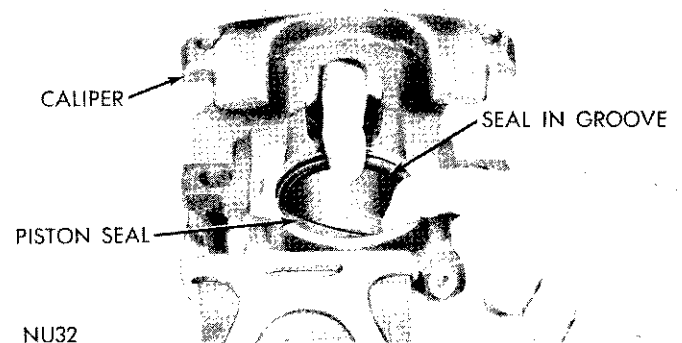
Fig. 15—Installing Piston Seal
