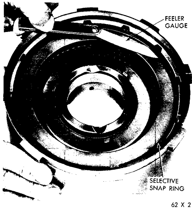
Fig. 74—Measuring Front Clutch Plate Clearance
