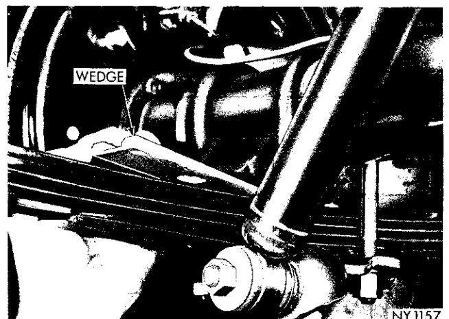
Fig. 9—Installing Tapered Wedge
