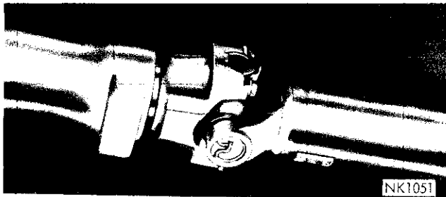
Fig. 14—Front Universal Joint—Single Cross Type (AY-1 Models)
