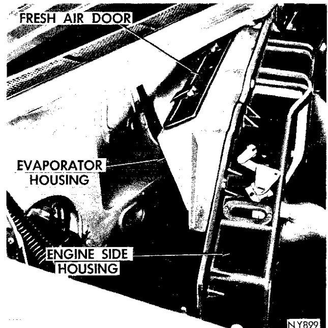
Fig. 46—Evaporator Installation Typical
