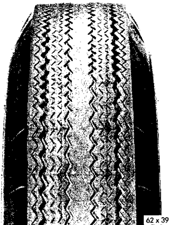
Fig. 11—Over Inflation Wear
