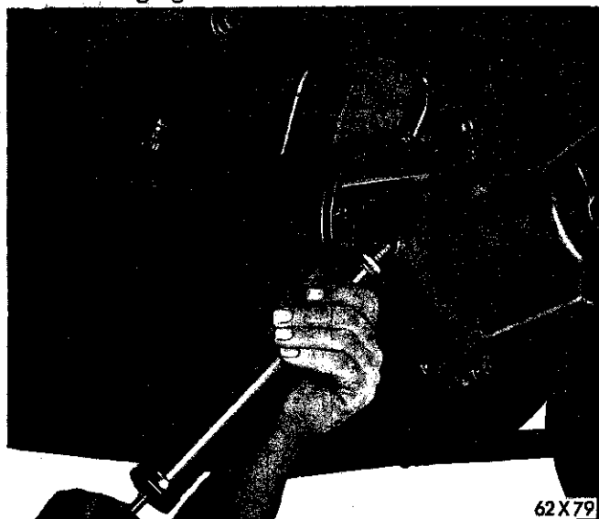
Fig. 22—Removing the Lubricant Using a Suction Tube
