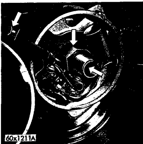
Fig. 15—Distributor Lubrication Points
