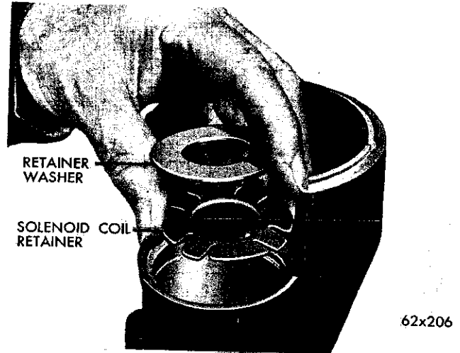
Fig. 9—Identification of the Solenoid Coil Retainer and Retainer Washer
