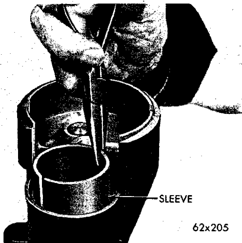
Fig. 8—Removing the Solenoid Coil Sleeve
