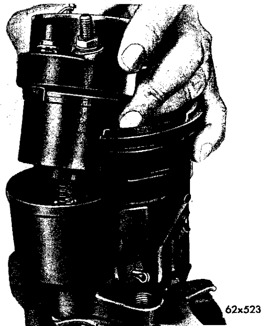
Fig. 23—Installing the Solenoid Coil, Sleeve and Brush Holder
