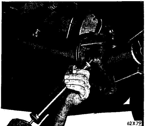
Fig. 22—Removing the Lubricant Using a Suction Tube
