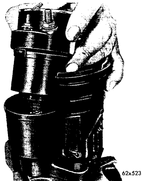
Fig. 41—Installing Solenoid Coil, Sleeve and Brush Holder
