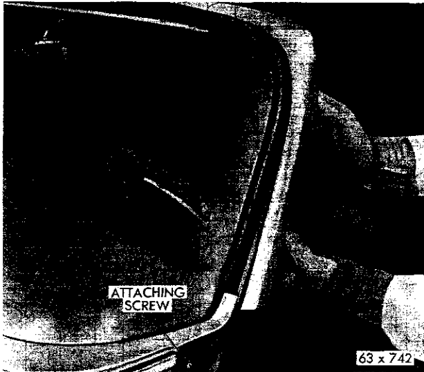
Fig. 62—Removing or Installing Windshield Moulding
