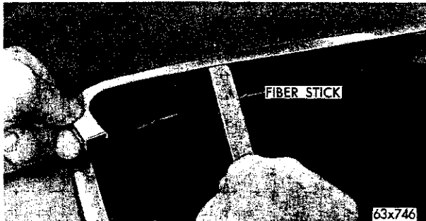
Fig. 71—Removing the Rear Window Upper Moulding
