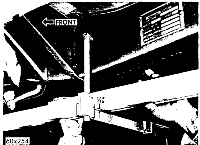
Fig. 17—Checking Body to Frame Alignment
