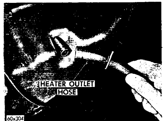
Fig. 7—Water Valve Test
