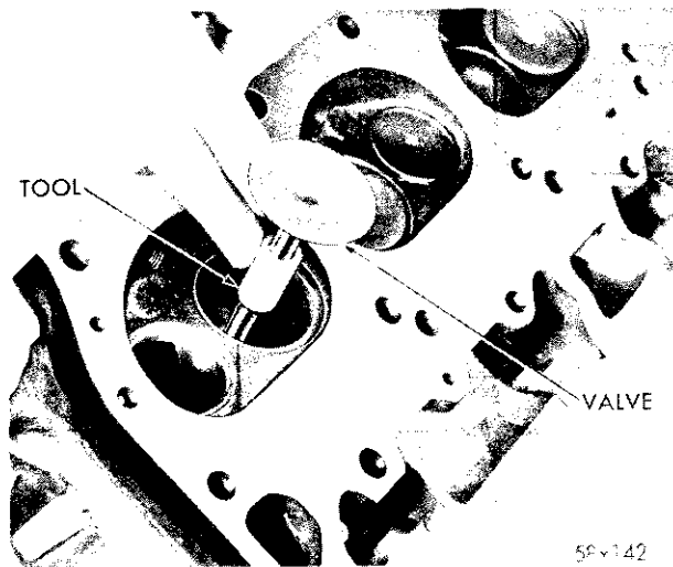
Fig. 13—Measuring Valve Stem Guide Clearance Using Tool C-3026
