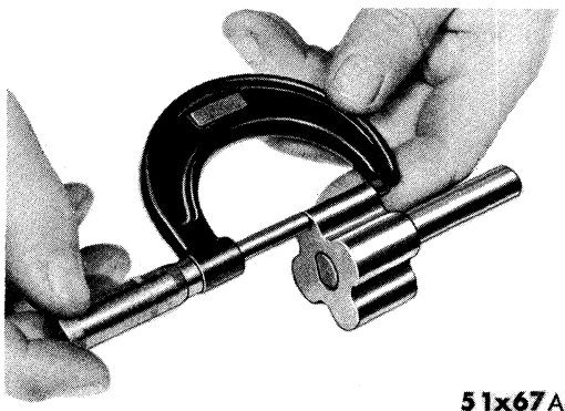
Fig. 92 — Measuring Inner Rotor Thickness
