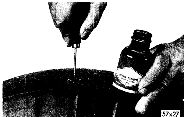
Fig. 6—Lubricating Puncture with Cement
