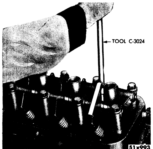
Fig. 22—Compressing Valve Spring (FirePower) (Typical of SpitFire)
