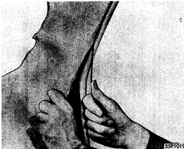
Fig. 93—Removing Headlining with Stiff Wire
