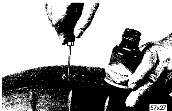
Fig. 5—Lubricating Puncture with Cement
