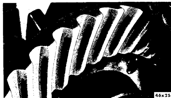
Fig. 37—Correct Gear Tooth Contact
