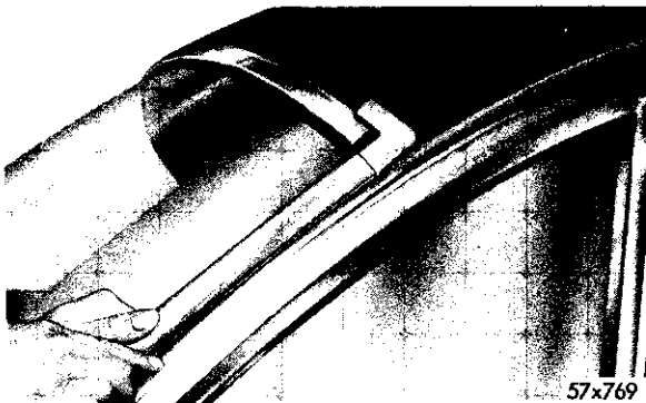
Fig. 64—Removing Rear Window Chrome Mouldings
