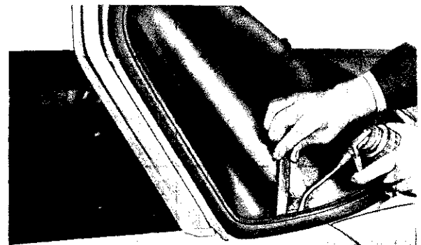
Fig. 6—Sealing Weatherstrip with Sealer Gun
