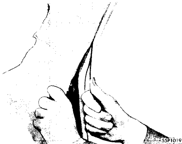
Fig. 80—Removing Headlining with Stiff Wire
