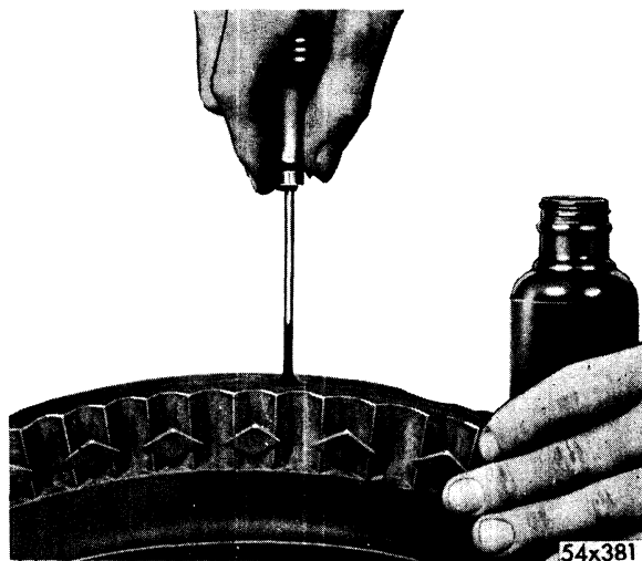
Fig. 10—Lubricating Puncture with Cement
