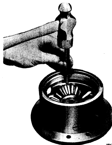
Fig. 22—Removing Differential Pinion Shaft Lock Pins
