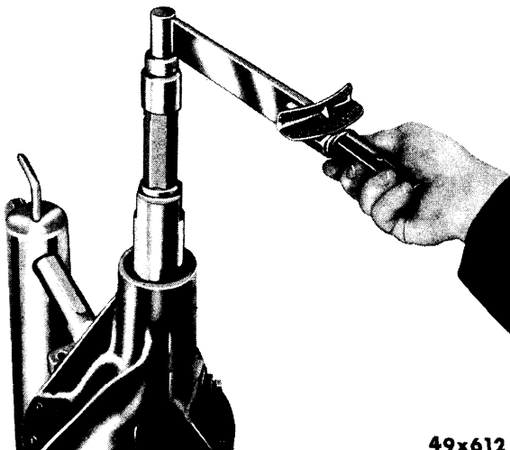
Fig. 36—Checking Torque Required to Turn Main Body
