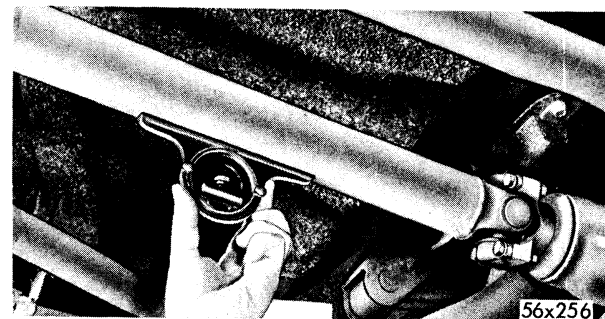
Fig. 16—Checking Rear Propeller Shaft Angles
