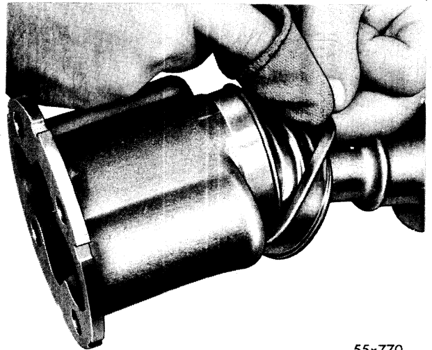
Fig. 11—Cleaning Lubricant from Contacting Surface of Dust Cover
