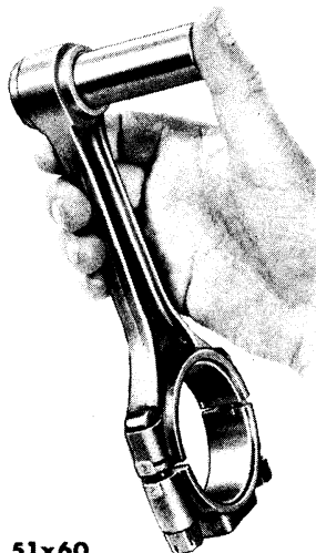
Fig. 46—Fitting Piston Pins in Connecting Rod
