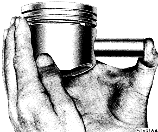
Fig. 47—Fitting Piston Pins in Piston (Typical)
