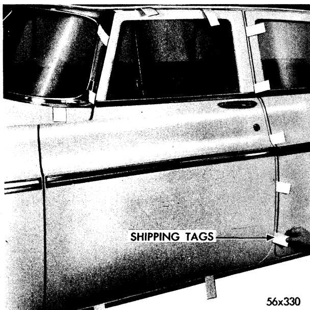
Fig. 16A—Checking Seal of Door
