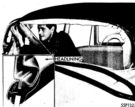
Fig. 98—Pressing Material onto Cemented Surfaces
