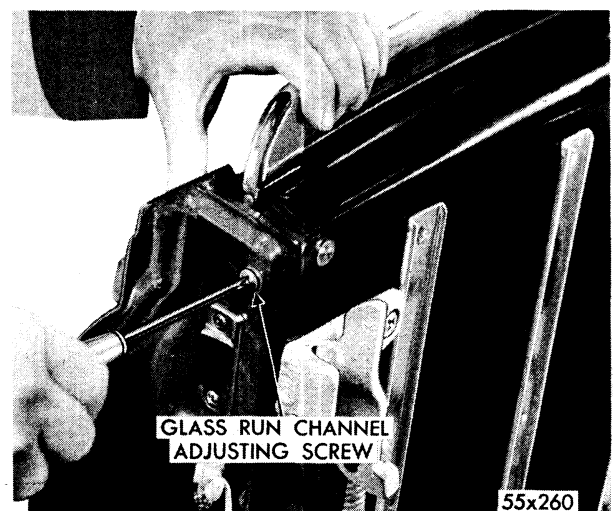
Fig. 76—Adjusting Glass Run Channel
