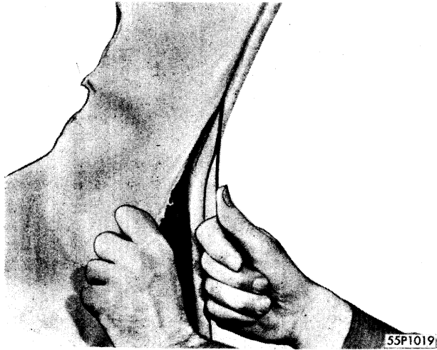
Fig. 87—Removing Headlining with Stiff Wire
