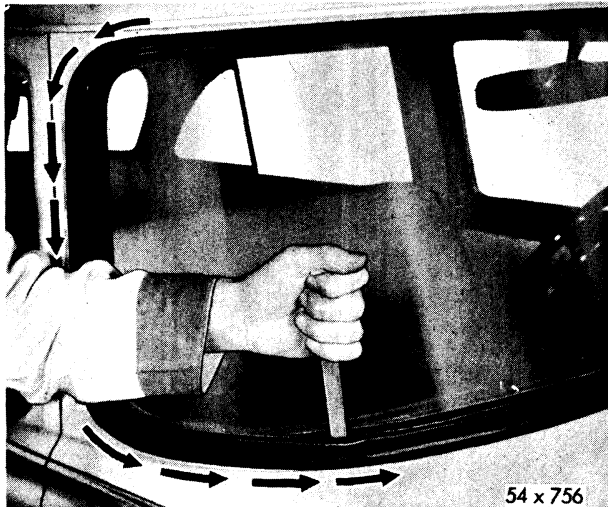
Fig. 51—Stripping Glass in Weatherstrip
