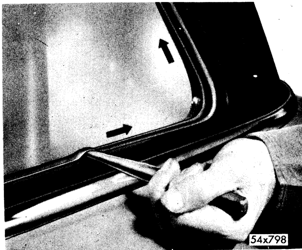
Fig. 84—Positioning Lip of Weatherstrip in with Wedge
