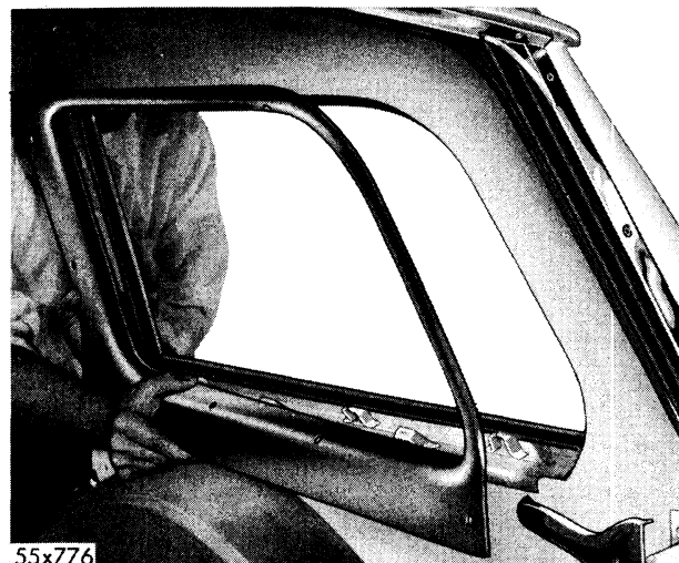
Fig. 79—Removing Garnish Moulding
