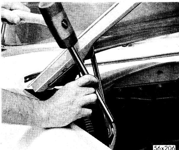
Fig. 13—Adjusting Hood (Forward)
