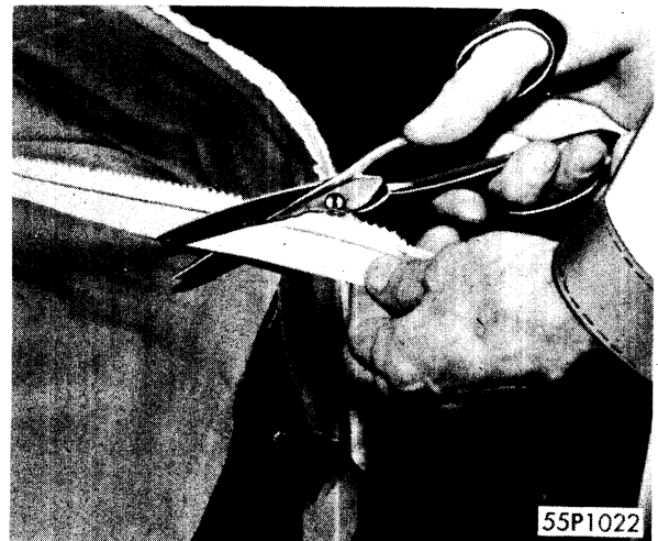
Fig. 90—Trimming Excess Listings even with Edges of Headlining
