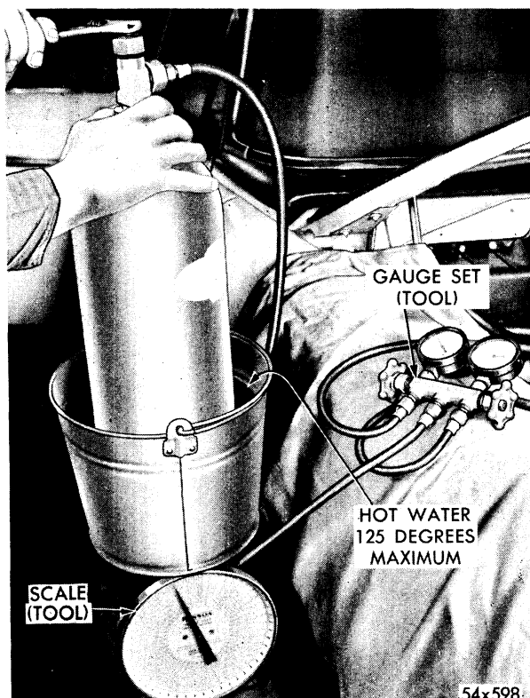
Fig. 6—Charging System with Freon 12
