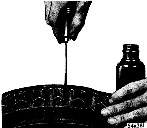
Fig. 11—Lubricating Puncture with Cement
