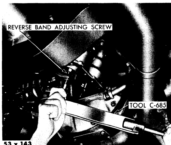
Fig. 39—Adjusting Reverse Band
