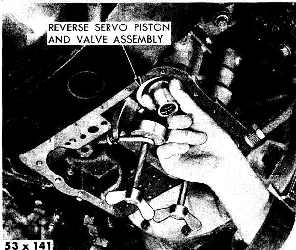
Fig. 46—Removal or Installation of Reverse Servo Piston and Valve Assembly
