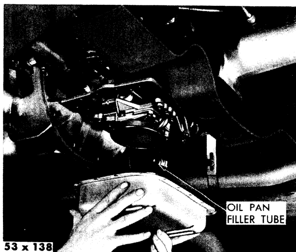
Fig. 40—Removing or Installing the Transmission Oil Pan
