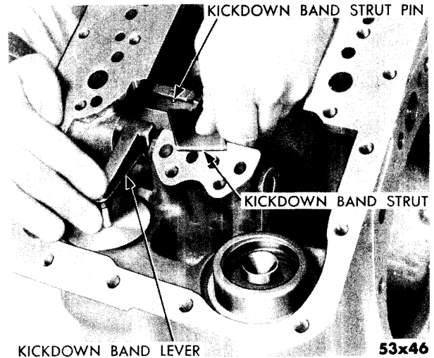
Fig. 109—Installation of Kickdown Band Strut
