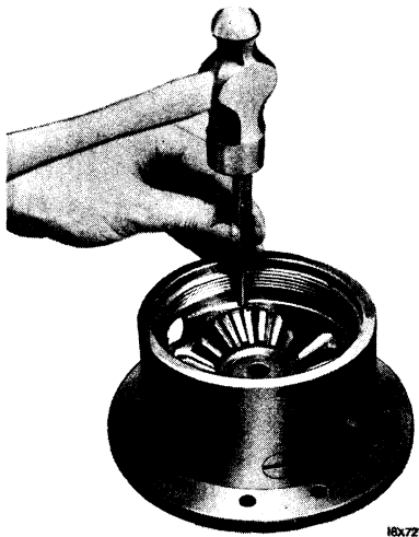
Fig. 23—Removing Differential Pinion Shaft Lock Pins
