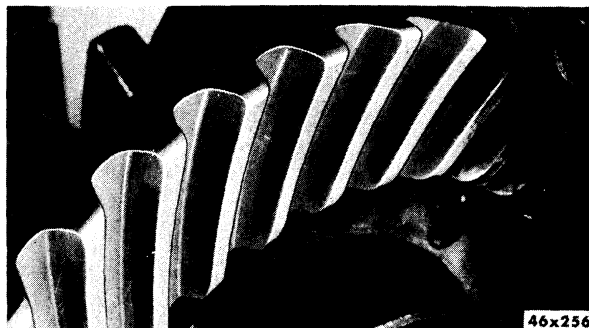
Fig. 46—Correct Gear Tooth Contact
