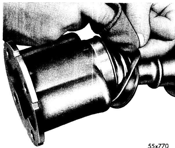
Fig. 11—Cleaning Lubricant from Contacting Surface of Dust Cover
