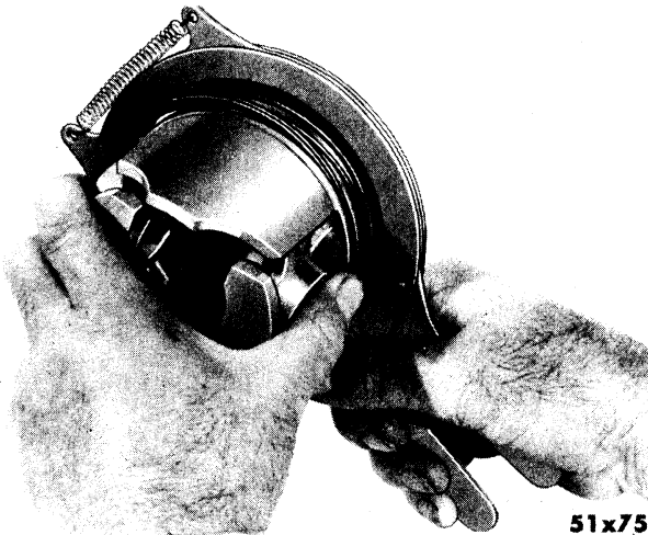
Fig. 113—Removing or Installing Piston Rings (Tool C-469)
