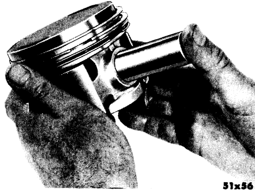
Fig. 115—Fitting Piston Pin In Piston
