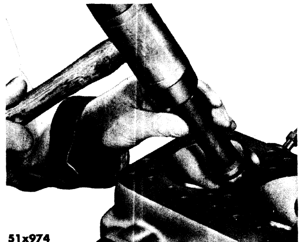
Fig. 145—Installing New Valve Seat Insert (Tool C-767)
