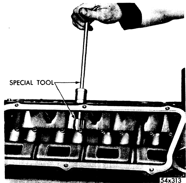
Fig. 93—Reaming Tappet Bores (Typical)
