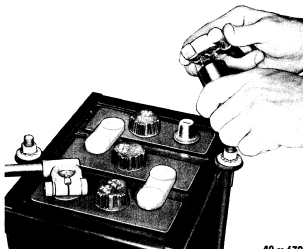
Fig. 30—Cleaning Inside of Cable Clamp (With Wire Brush Tool MX-75)
