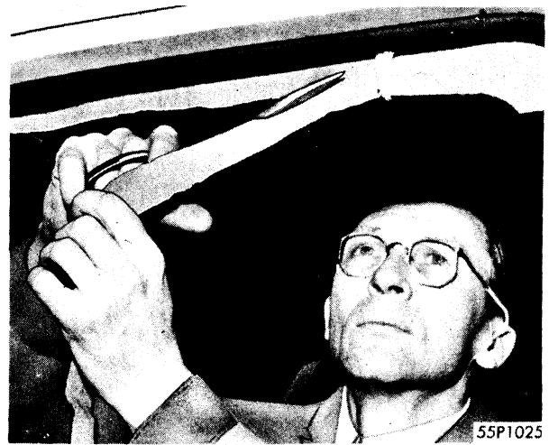
Fig. 89—Trimming Excess Material From Windcord
