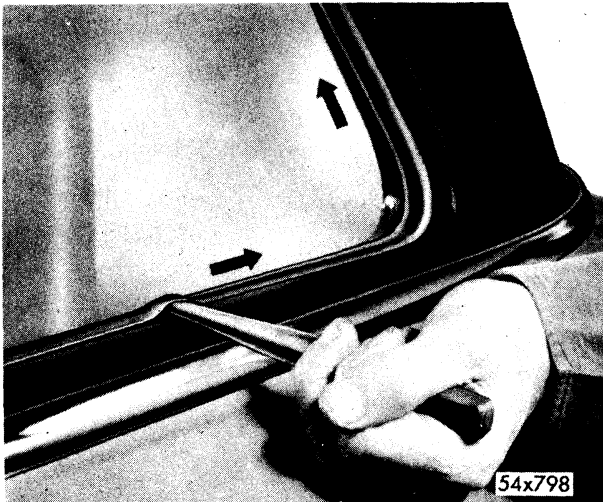
Fig. 80—Positioning Lip of Weatherstrip in With Wedge
