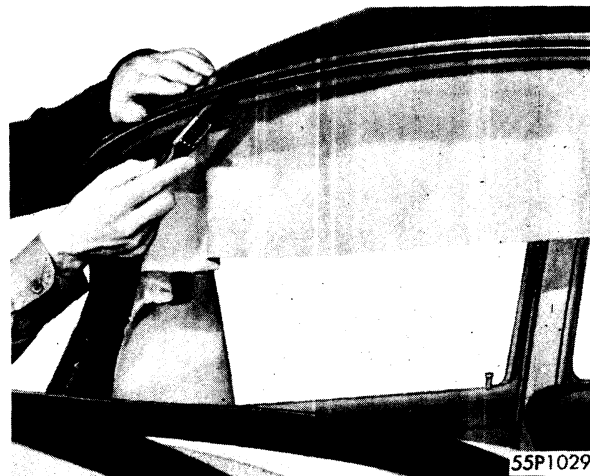
Fig. 92—Securing Material to Side Rails On Special Club Coupe
