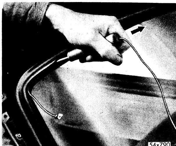
Fig. 57—Installing Pull Cord (Upper)
