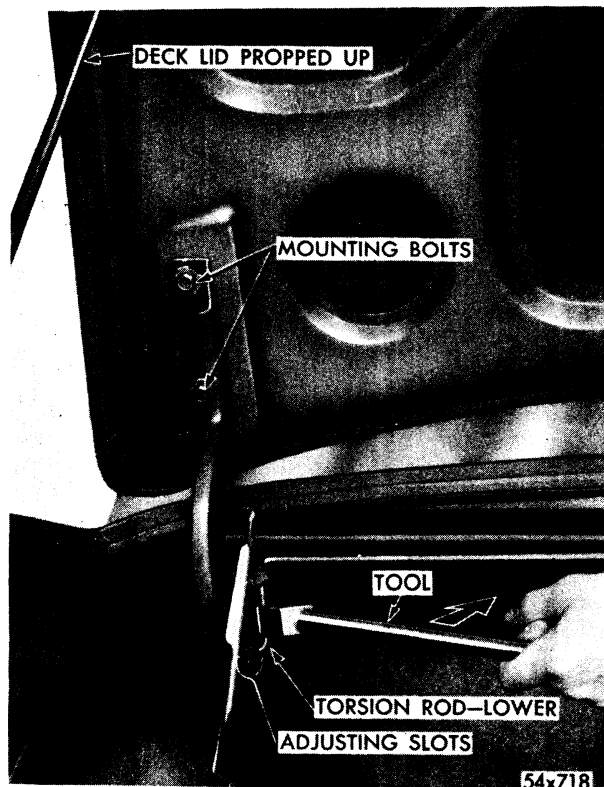
Fig. 20—Adjusting Torsion Bar Tension
