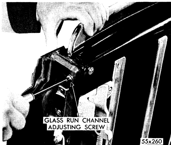
Fig. 72—Adjusting Glass Run Channel
